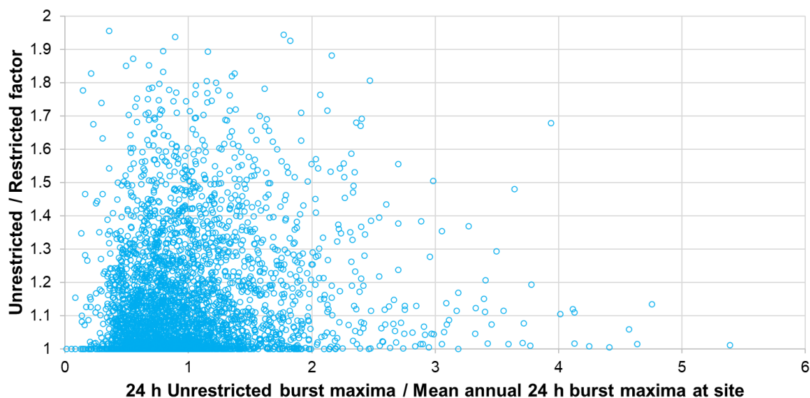
Figure 5-10 Relationship between U/R factor for 24 hour/1 day duration and burst intensity (ratio of unrestricted burst maxima at the site to mean annual 24 hour burst maxima at the site)
