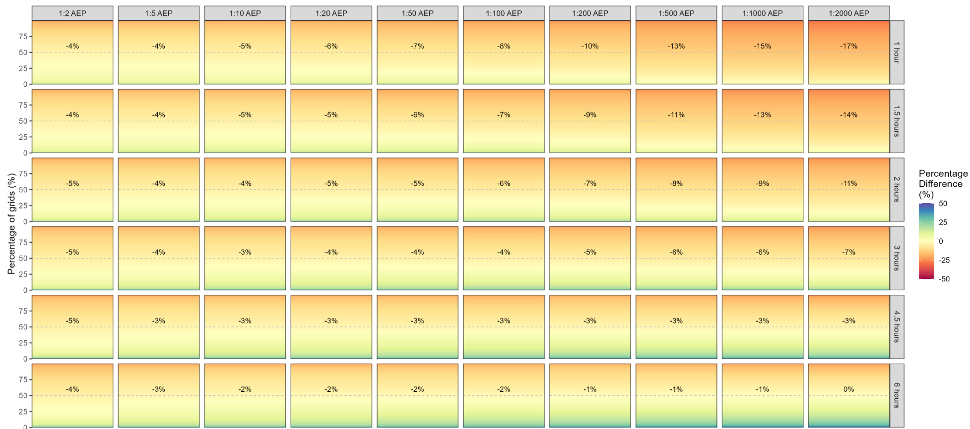
Figure J 2 Summary of percentage changes across different AEPs and durations (1 hour – 6 hours). The median change for the given durations and AEPs is displayed in the respective tiles.
