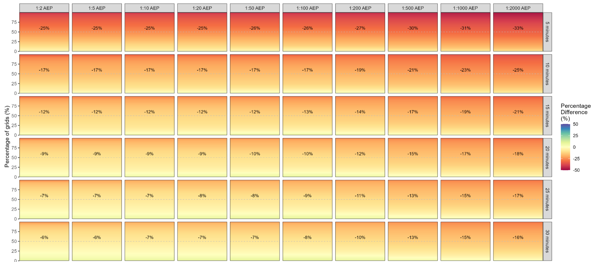
Figure J 1 Summary of percentage changes across different AEPs and durations (5 minutes – 30 minutes). The median change for the given durations and AEPs is displayed in the respective tiles.
