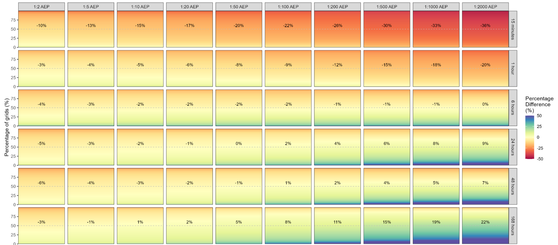
Figure 13-5 Summary of percentage changes across different AEPs and durations. The median change for the given durations and AEPs is displayed in the respective tiles.
